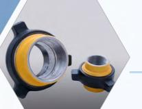
FLUXO Union Connections are made from Forged Alloy Steel. The steel has High Anti Corrosive property and High Strength. It comes with Weldon and Threaded type with all size from 1" to 12". From Sch 40 to 160 and in XXH type also. We provide all Sour Services Union Connections with Viton Seal Rings.
